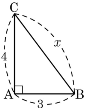
$$\overline{AB}^2 + \overline{AC}^2 = \overline{BC}^2$$
