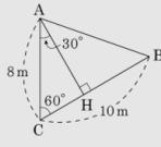
$$\overline{AH} = 8 \sin 60^\circ = 4\sqrt{3}(\text{m})$$
