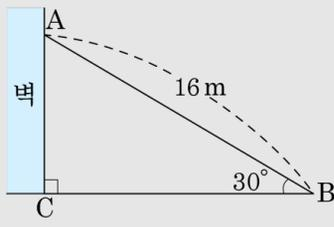
$$\begin{aligned}\overline{AC} &= 16 \sin 30^\circ \\ &= 16 \times \frac{1}{2} \\ &= 8(\text{m})\end{aligned}$$
