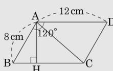
$$\overline{AH} = 8 \sin 60^\circ = 8 \times \frac{\sqrt{3}}{2} = 4\sqrt{3} \text{ (cm)}$$
