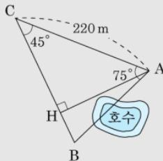
$$\overline{CH} = 220 \times \sin 45^\circ = 220 \times \frac{\sqrt{2}}{2} = 110\sqrt{2}(\text{m})$$
