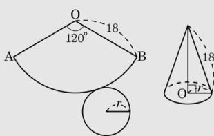
$$2\pi \times r = 2\pi \times 18 \times \frac{120^\circ}{360^\circ} \quad \therefore r = 6$$
